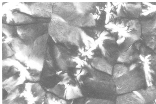
Figure 3 The spherulites of pure PEO cast from solution; the diagonal of the picture is 0.550 mm.
