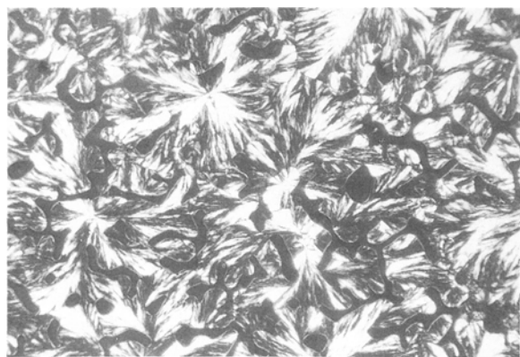
Figure 5 The PEO/PMMA blend cast from solution; the diagonal of the picture is 0.550 mm; 50 wt % PMMA.
