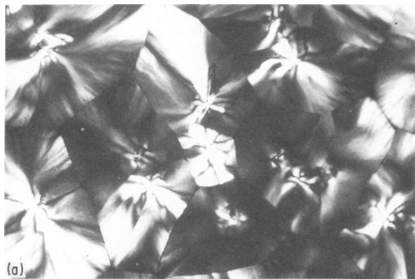
Figure 4 The PEO/PMMA blend cast from solution; the diagonal of the picture is 0.550 mm: (a) 10 wt % PMMA; (b) 30 wt % PMMA.
